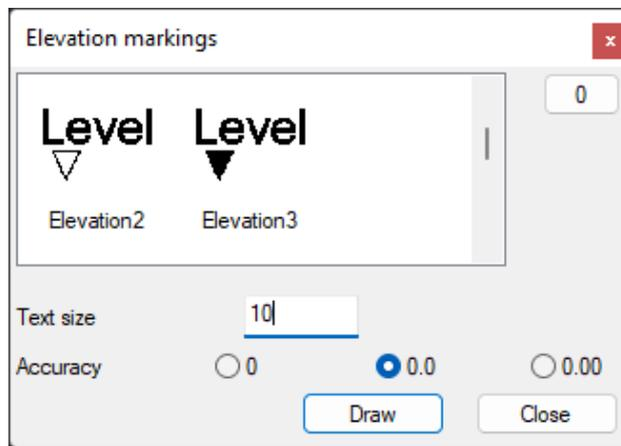
Elevation mark measures distance via Y axis from the beginning of the coordination system. You can click on 0 to set such a beginning.
