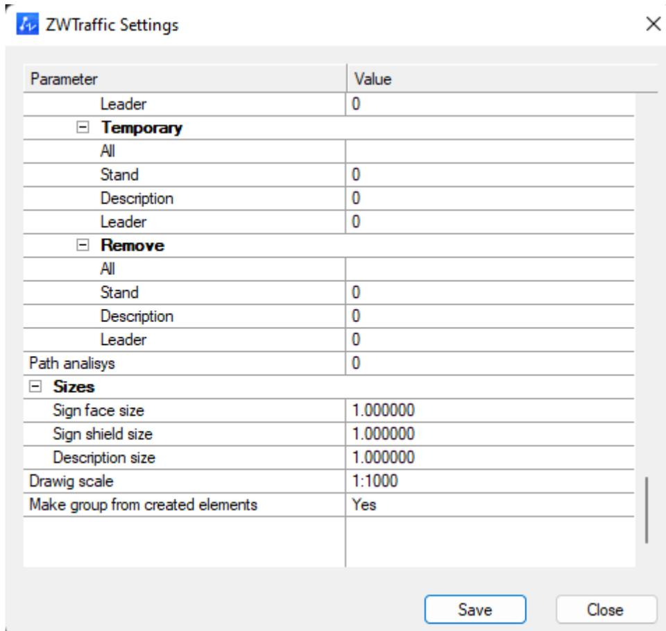
The default scale is set to 1:1000, but that can be changed, as well as for example state of signs. Every setting is saved to the file in directory: C:\Szansa\ZWTraffic\2025\EN\Configuration. There is a States.ini file, in which you can edit.
