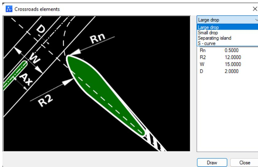
With Large and Small drop, you have to draw a line for its axis, then for the main road and the drop will be made. With Separating island and S-curve, pick a roundabout's outer line and click it. The entire structure will be made.
