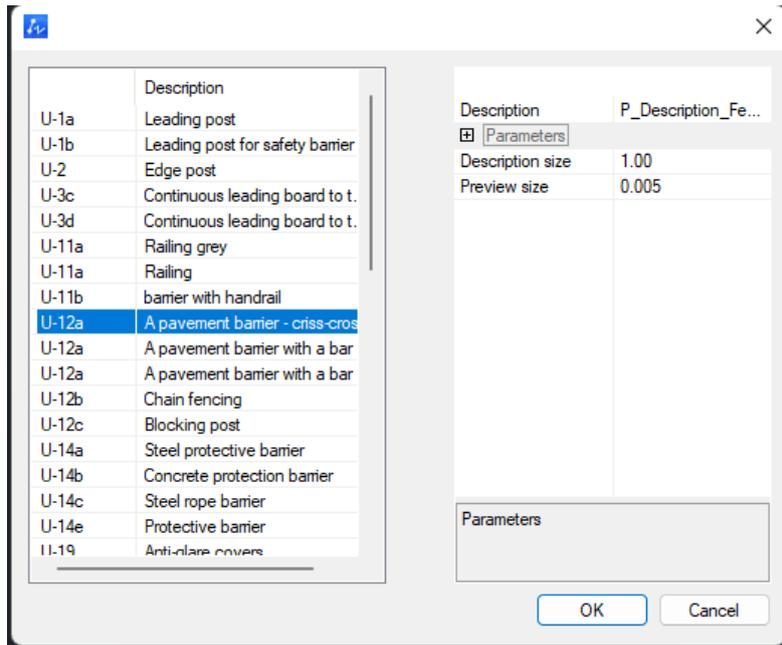
After that click on a line you want new barrier to be placed on and set its start and end.
