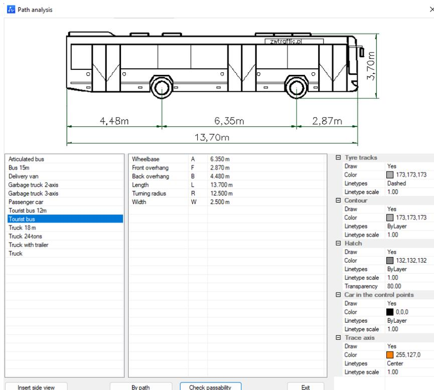
You can insert a side view of your car into the project. You can also choose a vehicle to test it, and there are two ways to do so.
