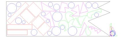
Objects that weren't fit into the selected area will be placed next to it. Furthermore, in the Command tab you will find information about the process of nesting.
